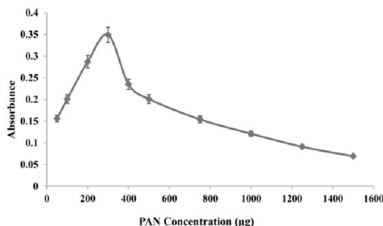
**Figure 5.** Effect of the PAN concentration on the MF-MSA-LLME procedure (concentration of Ag  $80 \mu\text{g L}^{-1}$ , pH= 12,  $\text{NaNO}_3$  concentration 0.1% w/v, extracting=  $200 \mu\text{L}$  PAN solution ( $\mu\text{g}$  in n-octanol), extraction time 2 min).
