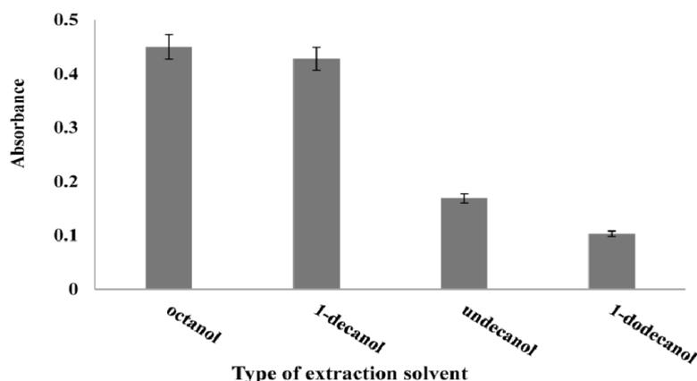
**Figure 2.** Effect of type of extraction solvent on the MF-MSA-LLME procedure (concentration of Ag  $80 \mu\text{g L}^{-1}$ , pH=12,  $\text{NaNO}_3$  concentration 0.1% w/v, extracting= 200  $\mu\text{L}$  PAN solution (300  $\mu\text{g}$  in extraction solvent), extraction time 2 min).
