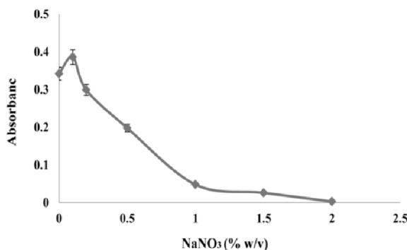
**Figure 7.** Effect salt on the MF-MSA-LLME procedure (concentration of Ag 80  $\mu\text{g L}^{-1}$ , pH= 12, extracting= 200  $\mu\text{L}$  PAN solution (300  $\mu\text{g}$  in n-octanol), extraction time 2 min).
