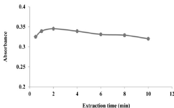
**Figure 6.** Effect of extraction time on the MF-MSA-LLME procedure (concentration of Ag 80  $\mu\text{g L}^{-1}$ , pH= 12,  $\text{NaNO}_3$  concentration 0.1% w/v, extracting= 200  $\mu\text{L}$  PAN solution (300  $\mu\text{g}$  in n-octanol)).
