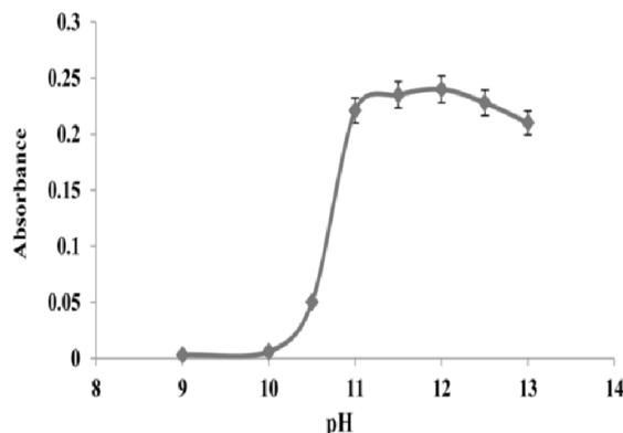
**Figure 4.** Effect of the pH of sample solution on the MF-MSA-LLME procedure (concentration of Ag  $80 \mu\text{g L}^{-1}$ ,  $\text{NaNO}_3$  concentration 0.1% w/v, extracting=  $200 \mu\text{L}$  PAN solution ( $300 \mu\text{g}$  in n-octanol), extraction time 2 min).
