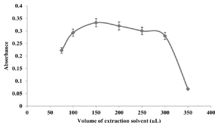
**Figure 3.** Effect of extraction solvent volume on the MF-MSA-LLME procedure (concentration of Ag  $80 \mu\text{g L}^{-1}$ , pH=12,  $\text{NaNO}_3$  concentration 0.1% w/v, extracting= PAN solution (300  $\mu\text{g}$  in n-octanol), extraction time 2 min).
