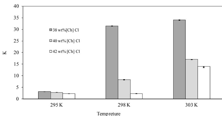
**Figure 4.** The effect of the temperature on the cephalixin partitioning in the aqueous two-phase system of [Ch]Cl+ K<sub>3</sub>PO<sub>4</sub>+H<sub>2</sub>O.
