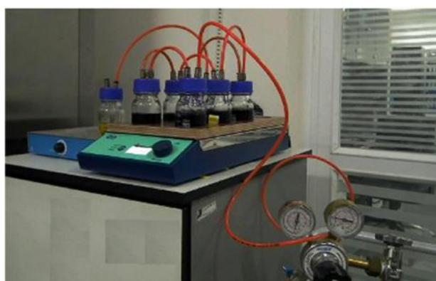
**Figure 6.** Dissolving cellulose in Cuen using magnetic stirrer under flushing with nitrogen.
