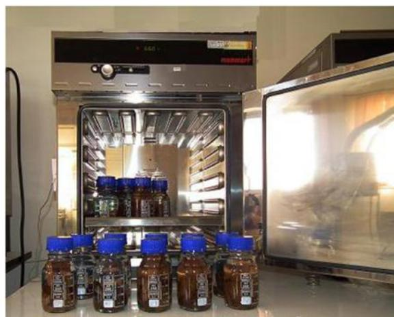
**Figure 4.** Containers including the samples ready to spend the accelerated pyrolysis in the 150°C.
