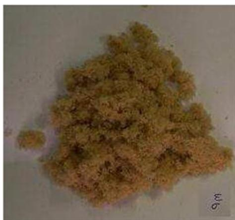
**Figure 5.** Degreased and fluffed cellulose.
