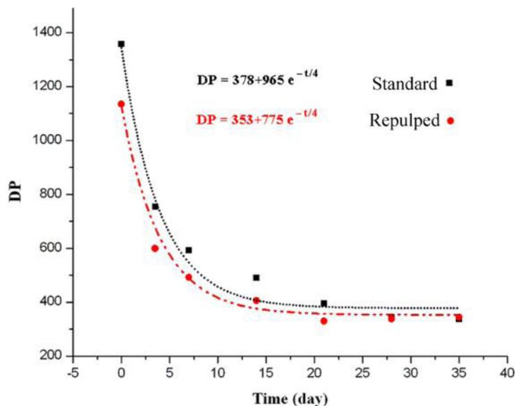
Figure 7. Comparative graphs of DP versus time for standard and repulped celluloses.
