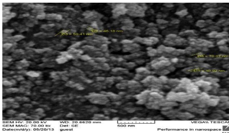
**Figure 2.** SEM image of  $\text{Fe}_3\text{O}_4$ .
