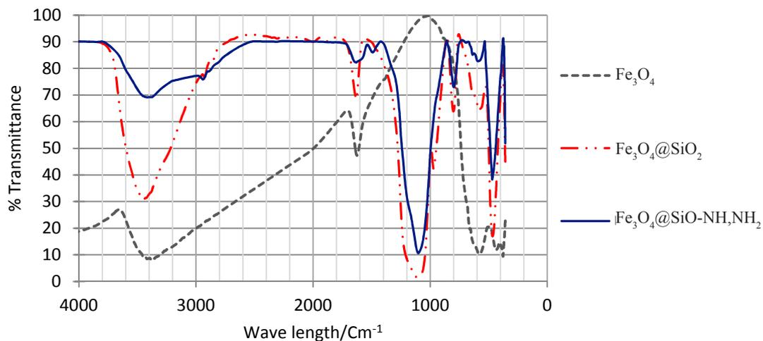
**Figure 4.** FT-IR spectra of  $\text{Fe}_3\text{O}_4$  and  $\text{Fe}_3\text{O}_4@SiO_2$  and  $\text{Fe}_3\text{O}_4@SiO_2$  core/shell modified by AEAPTMS.
