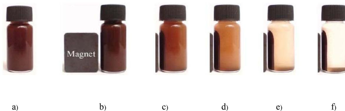
**Figure 9.** Digital photograph of the solution (a) dispersed magnetic  $\text{Fe}_3\text{O}_4@\text{SiO}_2\text{-AEAPTMS}$  particles and magnetic separation (b) using an external magnetic field after 0 min (c) 2 min (d) 3 min (e) 10 min (f) 30 min.
