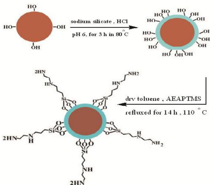
**Figure 1.** the Synthesis route of  $Fe_3O_4@SiO_2$ -AEAPTMS.
