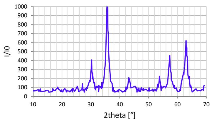
**Figure 3.** XRD pattern of  $\text{Fe}_3\text{O}_4$ .
