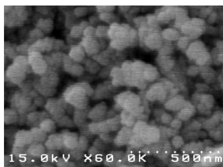
Figure 1. SEM image of NP-ZnO.
