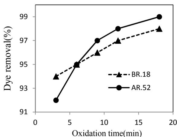
**Figure 4.** Comparative curve - Effect of time on the decolorization of BR.18 and AR.52 by Fenton process. Conditions: Initial volume of wastewater:50mL, Initial Concentration of dye: 50mg/L, Dose of  $H_2O_2$ :1.5g/ L, Concentration of  $Fe^{2+}$ :8mg/L, Mixing rate:200rpm.
