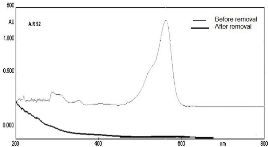
**Figure 6.** UV-vis absorbance spectra of A.R.52 (Comparative curve for before and after removal). Conditions: Initial concentration of dye solution: 50mg/L, Initial volume of wastewater:50mL, Volume of H<sub>2</sub>O<sub>2</sub>:1.5g/L, Concentration of Fe<sup>2+</sup>: 8(mg/L), Mixing rate :200rpm, Reaction time:18 min.
