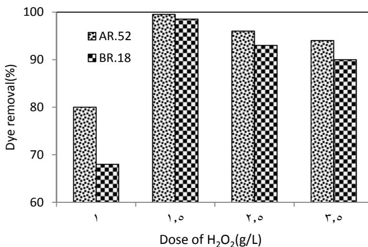
**Figure 3.** Comparative curve -Effect of  $H_2O_2$  dose on the decolorization percent of BR.18 and AR.52. Conditions: Initial Concentration of dye: 50mg/L, Initial volume of wastewater: 50mL, Initial pH:3, Concentration of  $Fe^{2+}$ : 8(mg/L), Mixing rate :200rpm.
