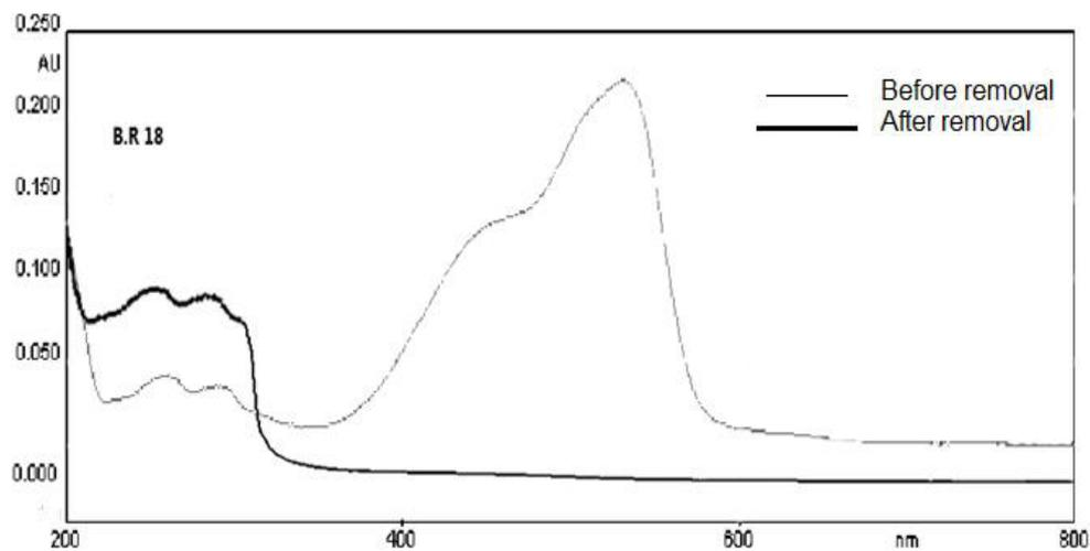
**Figure 7.** UV-vis absorbance spectra of B.R.18 (Comparative curve for before and after removal). Conditions: Initial concentration of dye solution: 50mg/L, Initial volume of wastewater:50mL, Volume of H<sub>2</sub>O<sub>2</sub>:1.5g/L, Concentration of Fe<sup>2+</sup>: 8(mg/L), Mixing rate :200rpm, Reaction time: 18 min.
