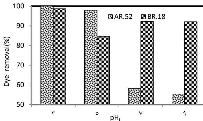
**Figure 2.** Comparative curve -Effect of initial pH on the dye removal efficiency percent of BR.18 and AR.52. Conditions: Initial Concentration of dye: 50mg/L, Initial volume of wastewater:50mL, Dose of H<sub>2</sub>O<sub>2</sub>:1.5g/L, Concentration of Fe<sup>2+</sup>:8mg/L, Mixing rate:200 rpm.
