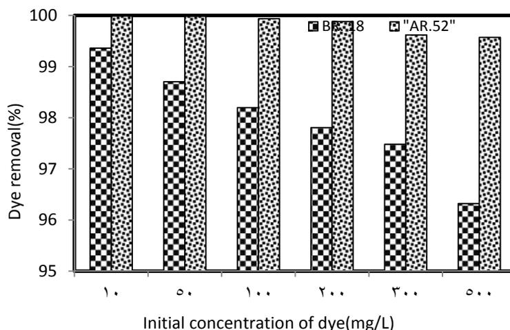
**Figure 5.** Comparative curve- Effect of initial dye concentration on the decolorization of BR.18 and AR.52. Conditions: Initial volume of wastewater: 50mL, Dose of  $H_2O_2$ : 1.5g/L, Initial pH: 3, Concentration of  $Fe^{2+}$ : 8 mg/L, Mixing rate: 200rpm.
