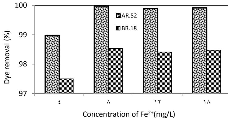
**Figure1.** Comparative curve - Effect of Fe<sup>2+</sup> concentration on the dye removal efficiency percent of BR.18 and AR.52. Conditions: Initial Concentration of dye: 50mg/L, Initial volume of wastewater:50mL, Dose of H<sub>2</sub>O<sub>2</sub>:1.5g/L, Mixing rate :200rpm, Oxidation time:18 Min.
